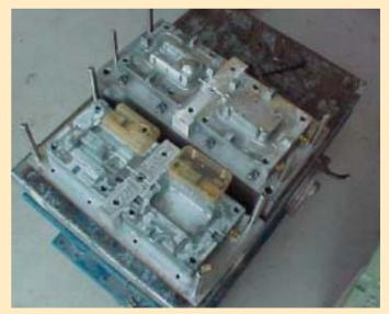
Cast kirsite cavity set for two parts molded together with SLA masters.
